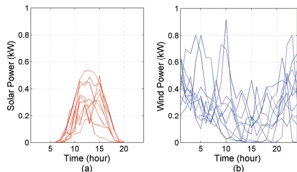
Fig. 2: Solar and wind power scenarios per 1kW capacity
